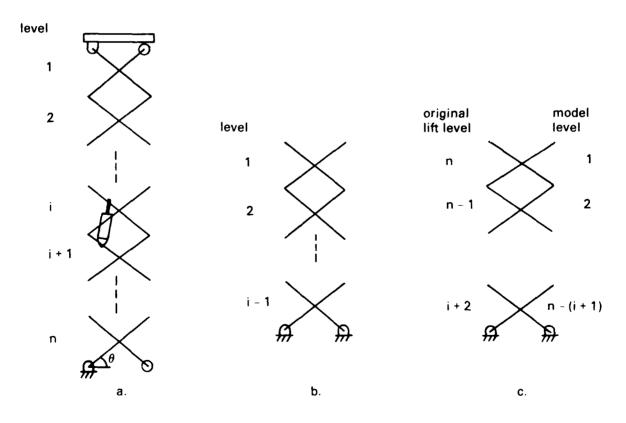
Figure 3. Scissor lift models.
