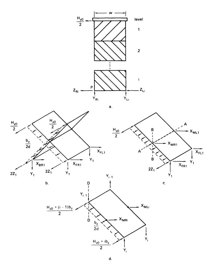
Figure 13. Freebody diagrams for load applied in the positive z direction.
