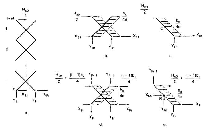
Figure 9. Freebody diagrams for load applied in x direction with the back joints pinned.
