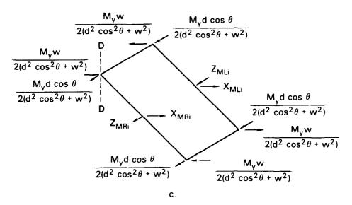
Figure 17. Freebody diagrams for an applied moment about the y axis (continued).
