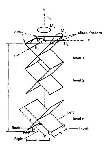
Figure 1. Nomenclature: applied loads and scissor lift dimensions.
