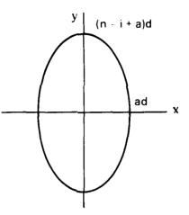
Figure 22. Path traveled by a point on a positively sloping scissor member.
