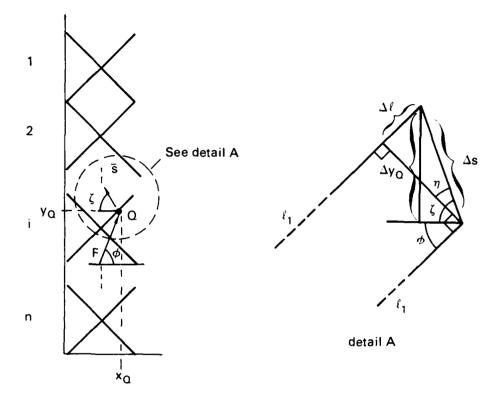
Figure 24. Actuator position and displacement nomenclature.
