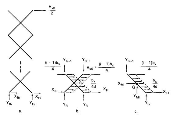
**Figure 10.** Freebody diagrams for load applied in the x direction with the front joints pinned. From figure 10c.
