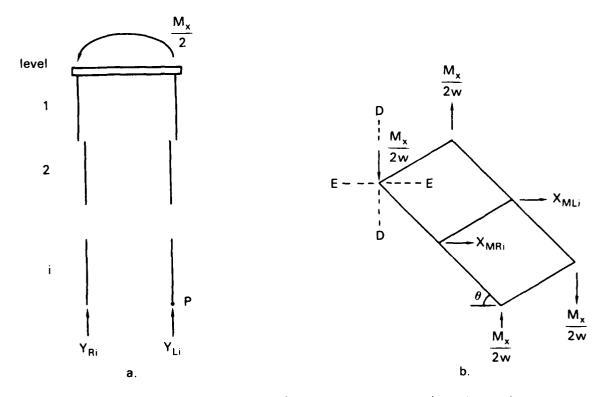
Figure 15. Freebody diagrams for an applied moment about the x axis.
