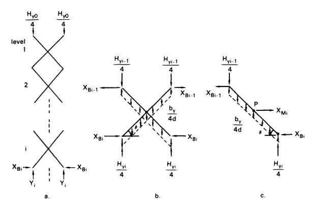
Figure 5. Freebody diagrams for load applied in the negative y direction.
