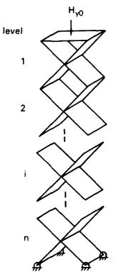
Figure 4. Basic scissor structure with load applied in the negative y direction.
