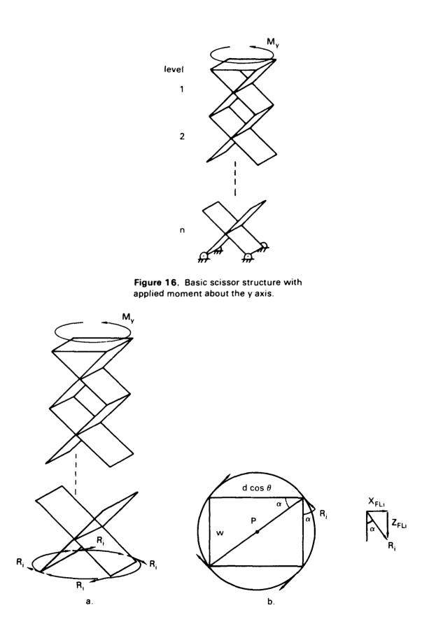
Figure 17. Freebody diagrams for an applied moment about the y axis.
