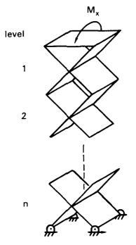
**Figure 14**. Basic scissor structure with applied moment about the x axis.
