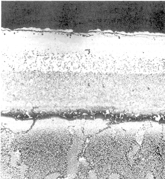
Figure 12. Micrograph of a Duplex Coating, GT-29+. (Bernstein and Allen, 1993)
