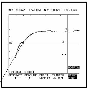
Notice the dimple in the upward slope of the waveform. This is caused from the pintle movement within the solenoid. This is a great test not only for verifying command, but also seeing that command, and the reaction that occurred.
