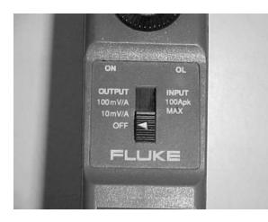
On most low amp probes there are two different settings to choose from, a 10 amp setting or a 100 amp setting. More often than not you will want to use the 100 amp setting. If you switch to the 10 amp scale many times the probe will be too sensitive. This will cause too much noise on your lab scope screen if you are trying to diagnose a very low amperage circuit.
