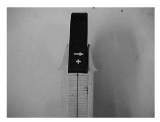
Most probes are directionally sensitive. What this means is, if you do not connect the probe over the wire in the proper direction, the waveform will display upside down. This will not damage the probe, but may lead you to believe that there is a problem when actually – there is not.
