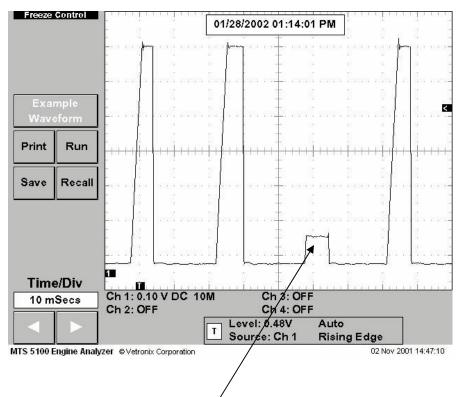
The module would build amperage up to approximately 1 amp before it would break down.
