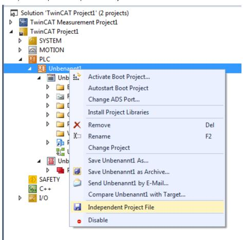
Objects that are saved as Independent Project Files are marked in the TwinCAT tree with the aid of an overlay icon in the form of a small floppy disk. A black floppy disk indicates that there are no unsaved changes yet for this object, whereas this is the case with a red floppy disk.
