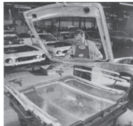
Fig. 29.13 A structural adhesive used to bond a stiffener to an aluminium car bonnet. To line up the two parts a purpose made fixture is designed
