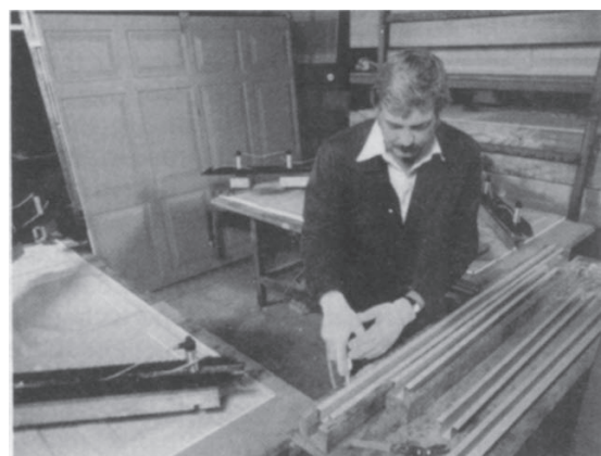
Fig. 29.14 Mild steel stiffeners are bonded to up and over garage door. Result: rigidity, unblemished exterior surfaces
