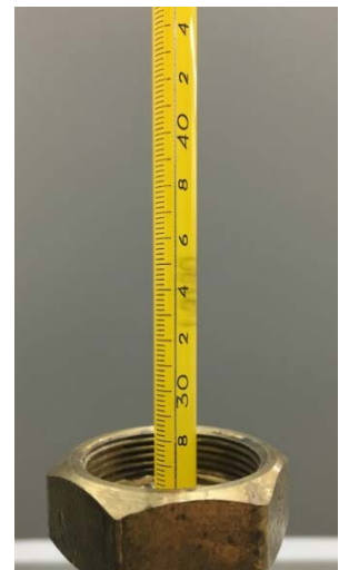
Figure B-2 - Total Immersion Thermometer Partially Immersed in a Thermowell
