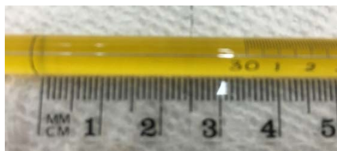
Figure B-5 - Measuring Between Immersion Ring and Start of Temperature Scale (34 mm)
