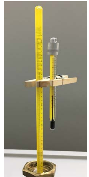
Figure B-4 - Measuring Temperature of the Emergent Liquid Column
