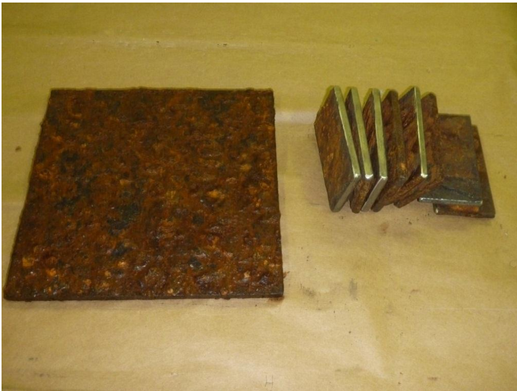
Figure 8. Test panels cut from ASTM Rust Grade D corroded 1/4 in. ASTM A36 steel plate, prior to surface preparation
