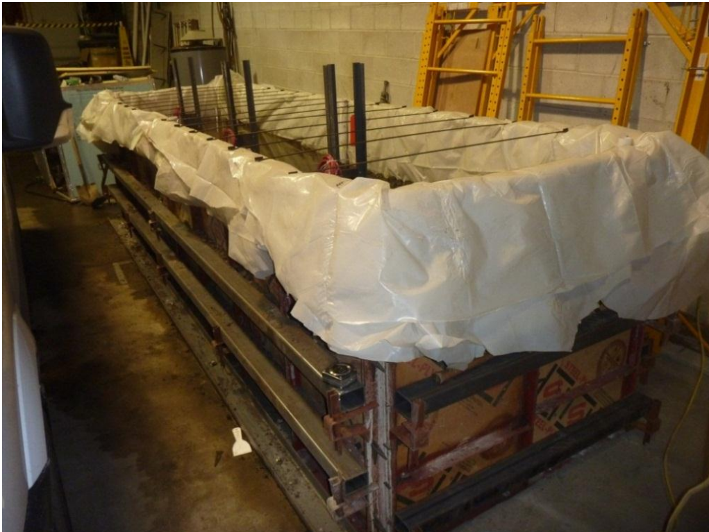
Figure 40. Soil tank for cathodic protection test
