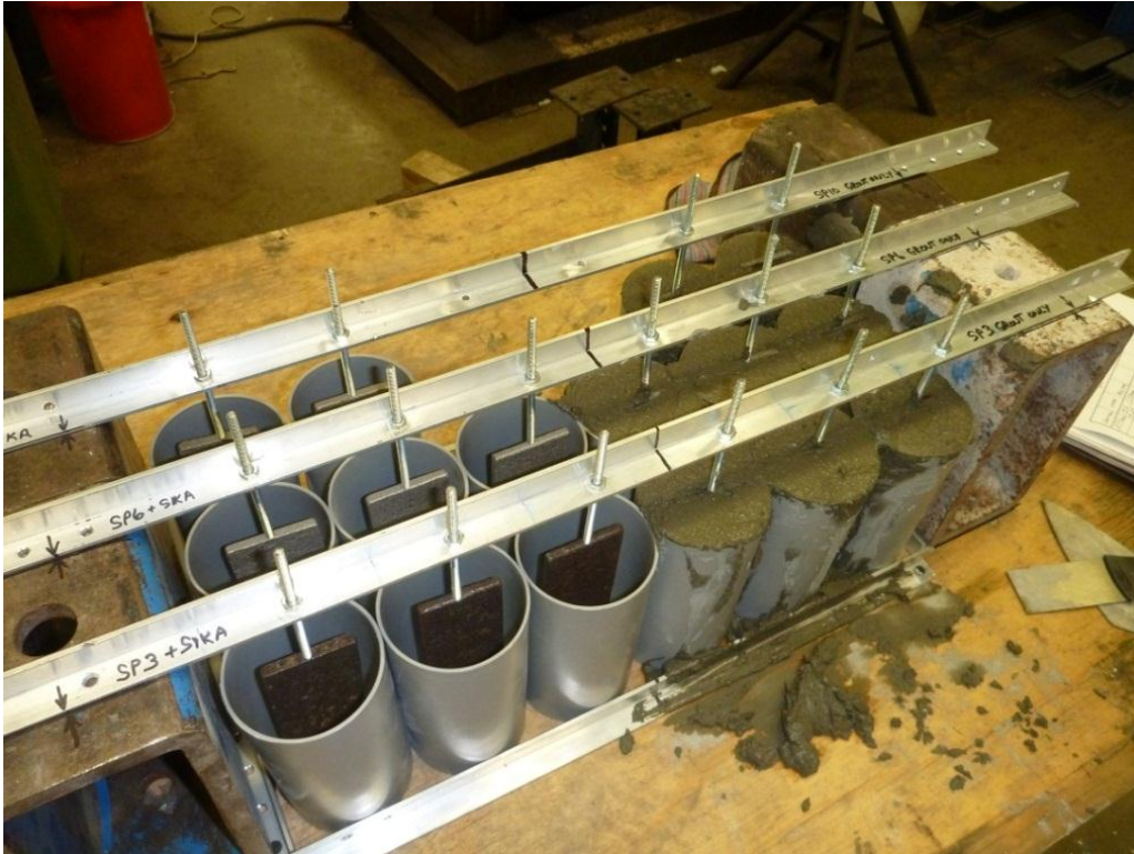
Figure 13. Formed grout encapsulation of test panels
