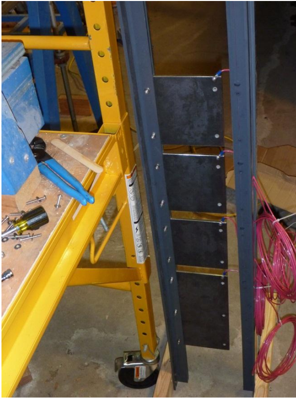
Figure 43. Partially assembled test pile.
