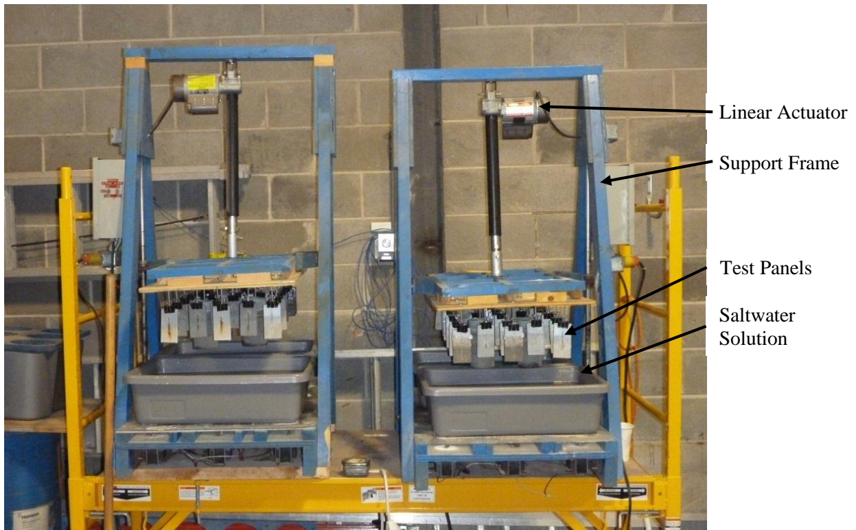
Figure 18. Cyclic immersion test setup
