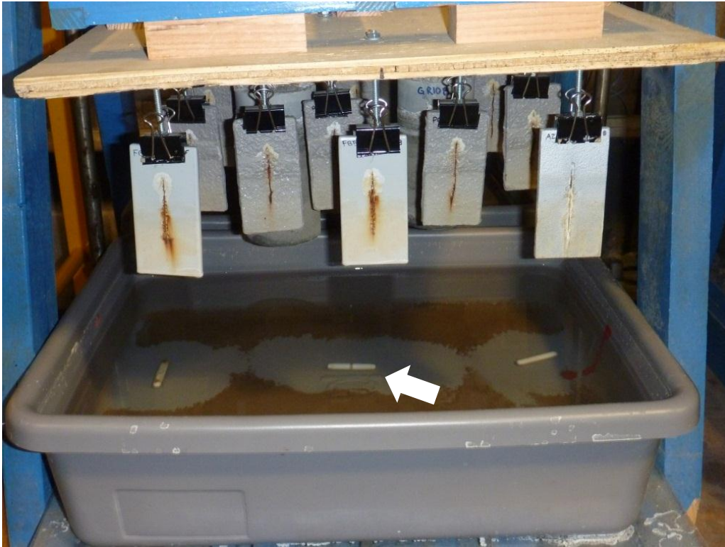
Figure 19. Close-up view of test panels. Arrow points to automatic stirrer.
