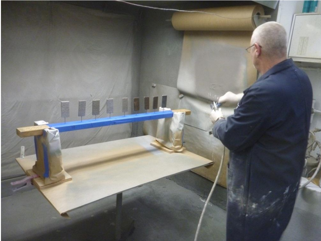
Figure 15. Spray application of glass flake polyester coating
