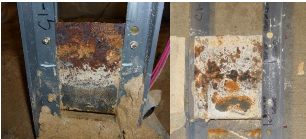
Figure 65. Plate 1 of Pile C before and after mortar block (top of sand is white line).
