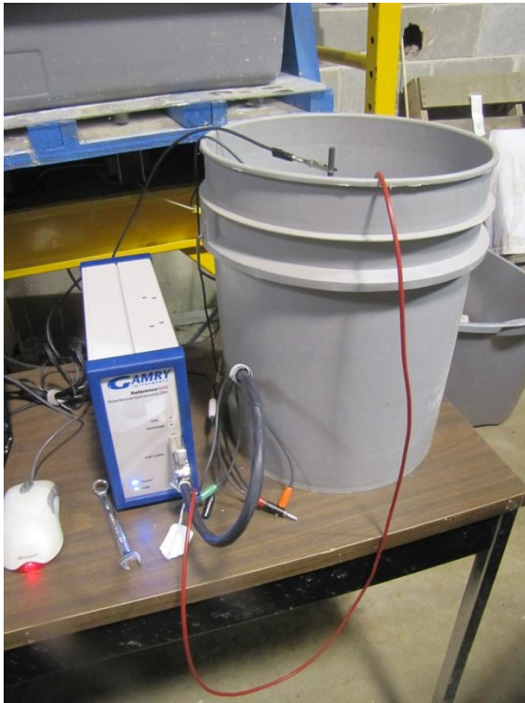
Figure 21. Test setup used for LPR and Potentiostatic EIS testing. Hidden from view in the grey bucket is a salt solution deep enough to submerge 50% of the coated specimen (working electrode), a Ag/AgCl reference electrode, and a graphite counter electrode. The Gamry unit to the left is a potentiostat used to control the tests.
