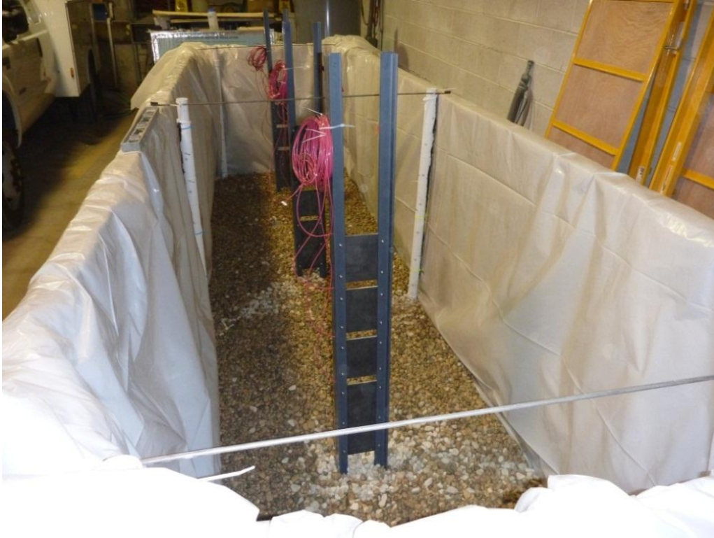
Figure 45. Test piles and gravel installed in soil tank. Note vertically oriented perforated PVC pipes for monitoring of water level during test.
