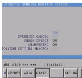
Automatic Running Monitor Displays the control status of each axis. Used to set ON / OFF for the machine lock function.
