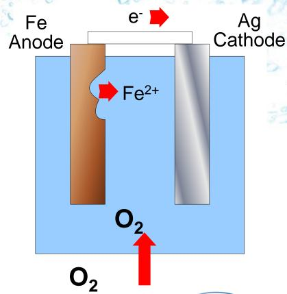
Oxygen is reduced to hydroxide at the cathode.
