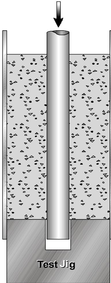
**Table 7** presents the 14-day shear bond strengths of the cement samples in the pipe-in-pipe and pipe-in-soft configurations. They were cured at atmospheric pressure in a water bath maintained at 45°F.
