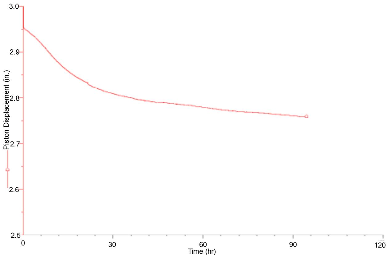
Changes in the cement volume are assumed to be overwhelmingly dominated by inner shrinkage, although any bulk shrinkage would also affect the volume. From the piston displacement data, the cement volume shrank by 6.8%.
