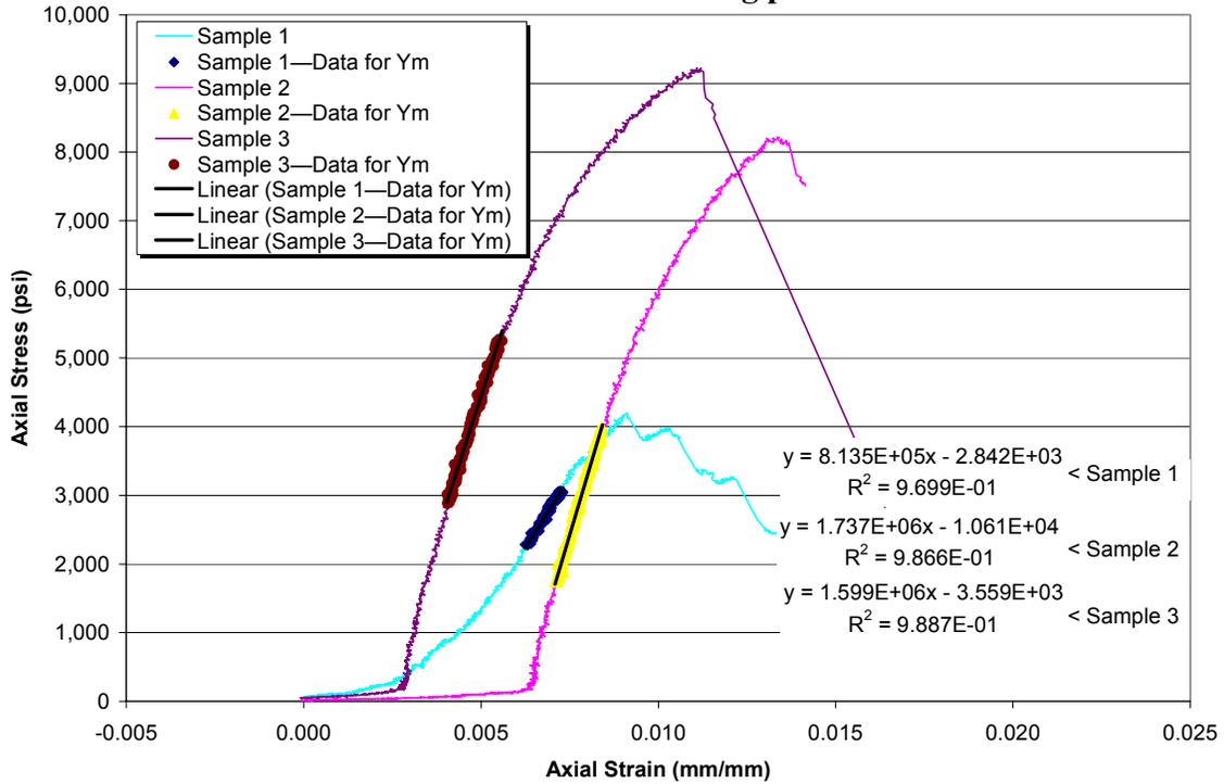
**Figure 3—Young’s modulus testing for samples cured in an unconfined condition and tested at a confining pressure of 1,500 psi**
