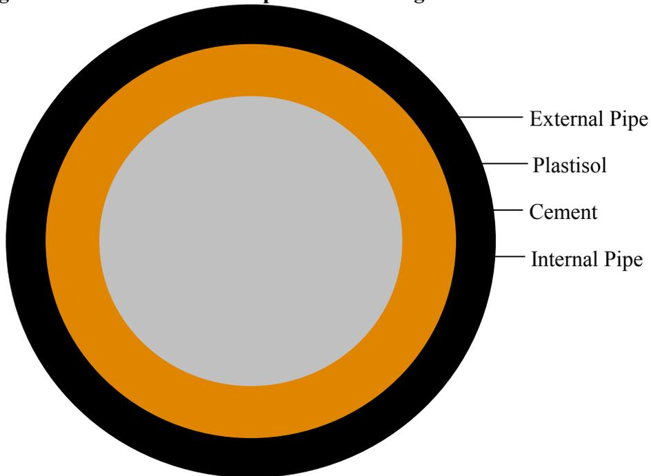
The shear bond measures the stress necessary to break the bond between the cement and the internal pipe. This was measured with the aid of a test jig that provides a platform for the base of the cement to rest against as force is applied to the internal pipe to press it through. (Figure 10) The shear bond force is the force required to move the internal pipe. The pipe is pressed only to the point that the bond is broken; the pipe is not pushed out of
