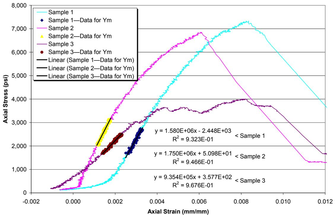
Tests were also conducted to determine the effect that temperature cycling has on Young's modulus. The temperature cycling procedure was designed to simulate temperature conditions that might be encountered during production of a well. The samples are first cured for 14 days in a 45°F water bath at atmospheric pressure. They are then subjected to five days of temperature cycling. During each of these five days of temperature cycling, the cured samples are cycled as follows.
