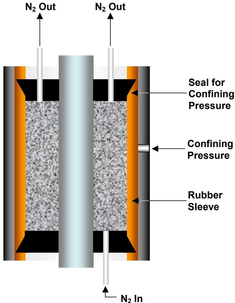
The inner pipe of the model will be the main conduit for the stressing medium. For instance, the inner pipe can contain heated fluids while the remainder of the system is at a different temperature; this simulates the hotter formation fluids that can be experienced during production. The inner pipe of the model can also be pressurized up to 5,000 psi, simulating casing pressure testing which is believed by many to lead to loss of annular seal because of the expanding and contracting casing.
