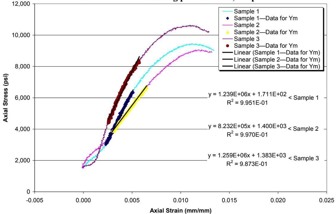
**Figure 4—Young’s modulus testing for samples cured in an unconfined condition and tested at a confining pressure of 5,000 psi**
