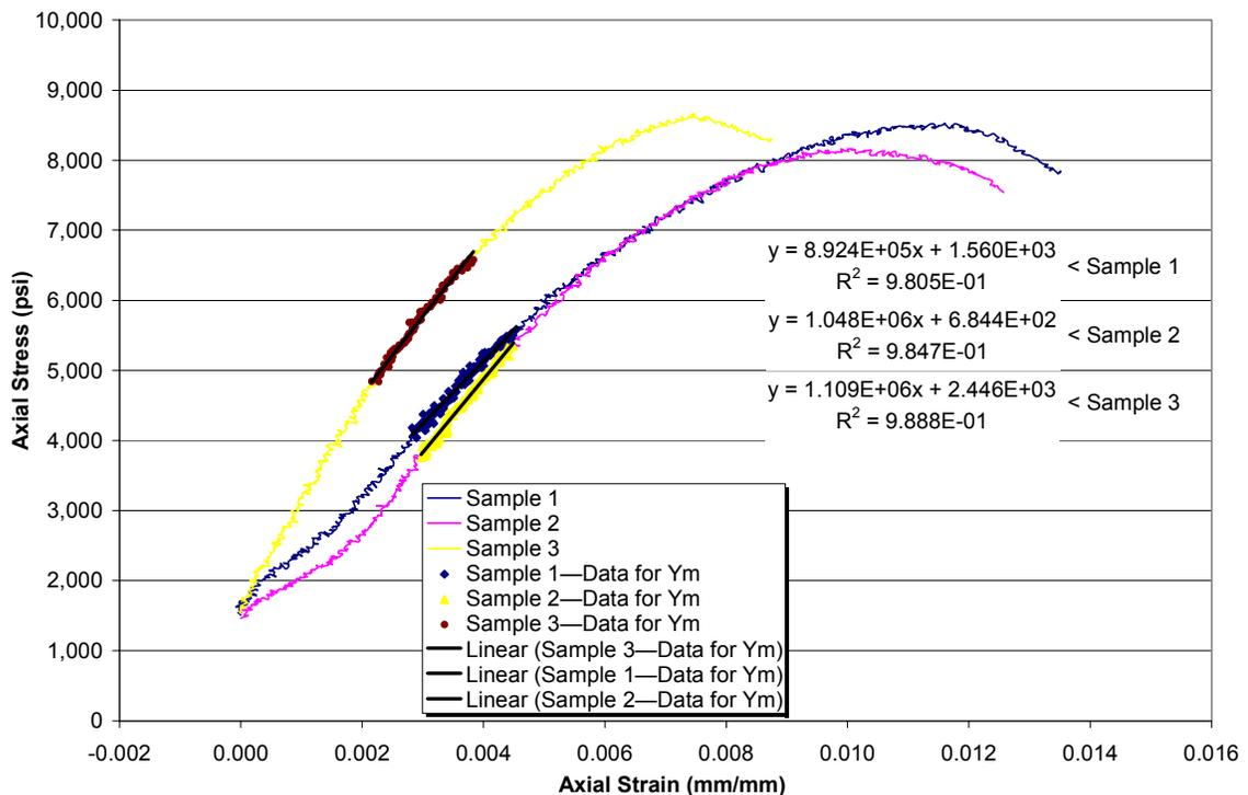
Some of the variation in the Young's modulus data could be attributed to settling of the cement slurry. The samples were cured in molds that were 10 in. long, and the individual 3-in. samples were then cut from the 10-in. specimens. For future testing, to avoid potential slurry settling, the slurry will be preconditioned for 20 minutes in an atmospheric consistometer and then poured into individual, shorter molds so only one individual test sample will come from each mold.
