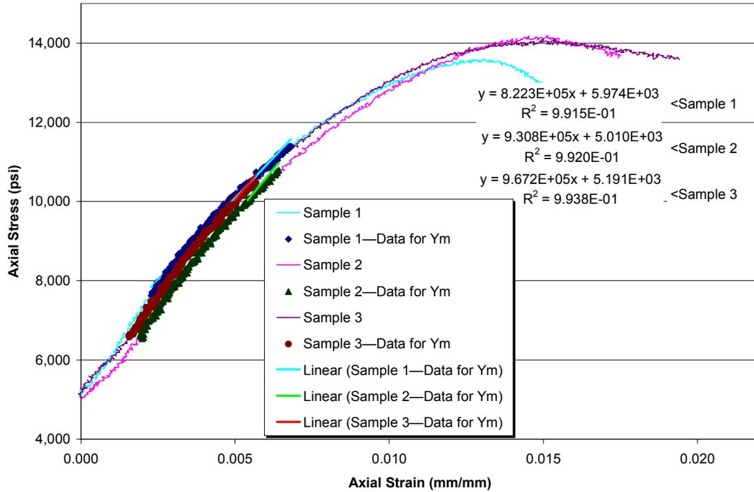
**Figure 5—Young’s modulus testing for samples cured in a confined condition and tested at zero confining pressure**
