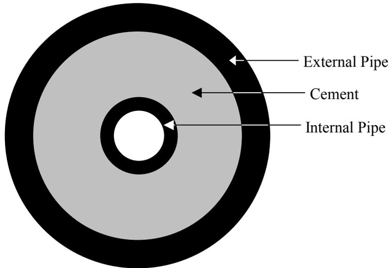
**Figure 9— Cross-Section of Pipe-in-Soft Configuration for Shear Bond Tests**
