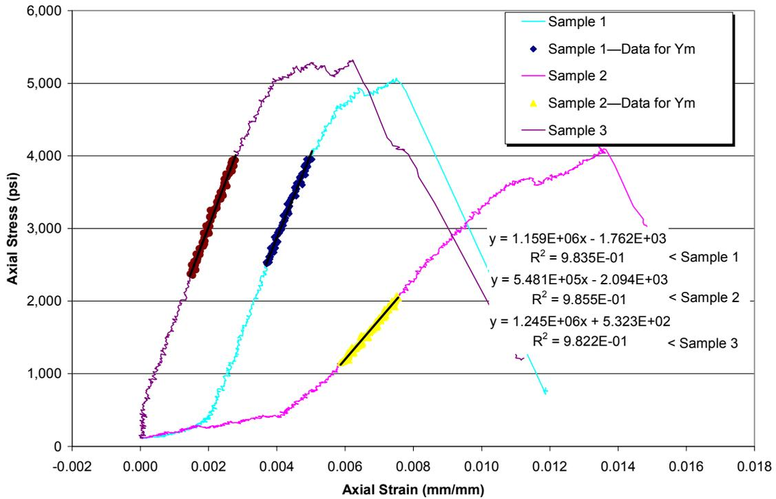
**Figure 7—Young’s modulus testing for samples cured in an unconfined condition and then temperature-cycled for five days and tested at a confining pressure of 1,500 psi**
