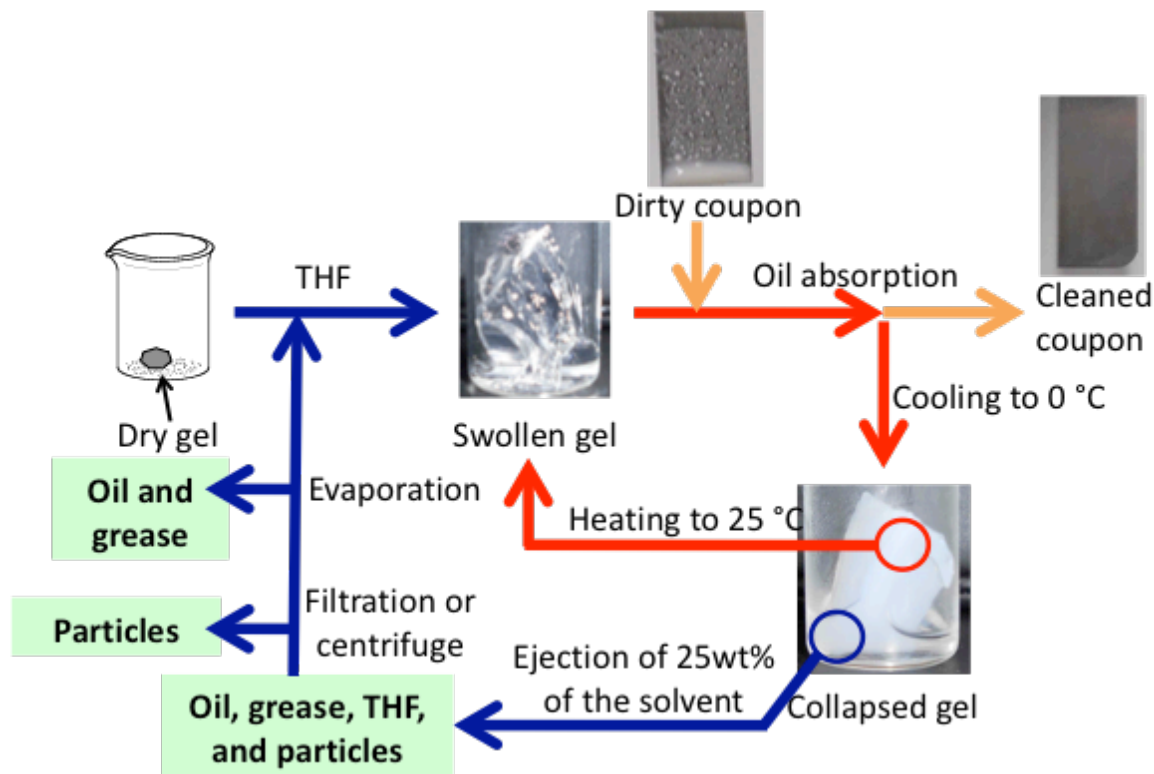
Figure 20. Cyclic surface cleaning process with swollen NG-18-1% gel in THF
