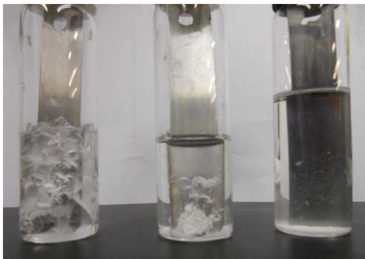
Figure 23. Photographs metal coupon immersed in gels: (left) NG-18-1%, (center) NG-18-0.5%, and (right) toluene
