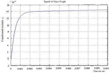
Fig. 13. Time Response of  $y_2$  for the linearized system in closed loop when  $v_1 = 30$ ;  $k_v = 50$ ;  $k_i = 2$
