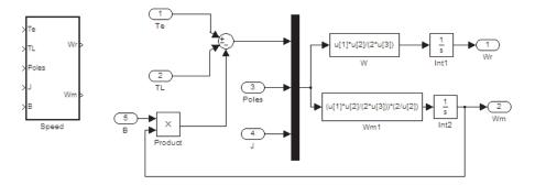
Fig. 7. Speed Block in Simulink
