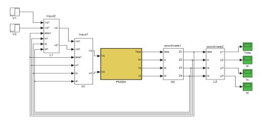
Fig. 9. Linearization of PMSM model
