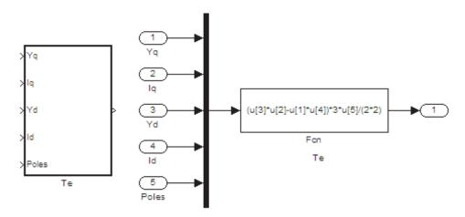
Fig. 6. T<sub>e</sub> Block in Simulink
