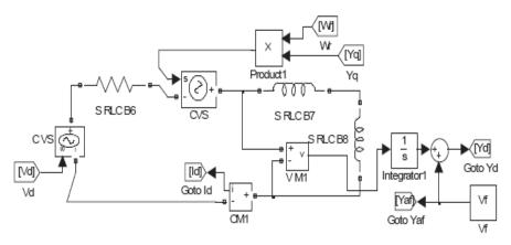
Fig. 5. d-axis circuit
