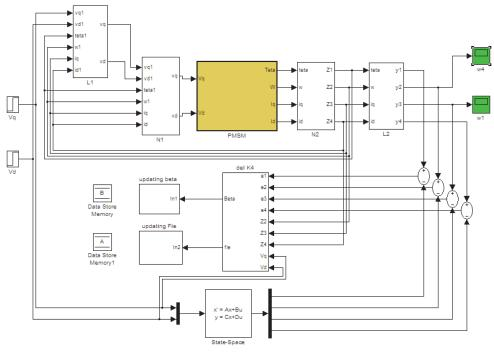
Fig. 18. Simulation diagram including controller tuning
