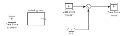
Fig. 16. Updation rule using Memory Read and memory Write Blocks
