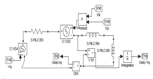
Fig. 4. q-axis circuit
