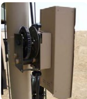
Winch power unit for EX- and EXL-masts
