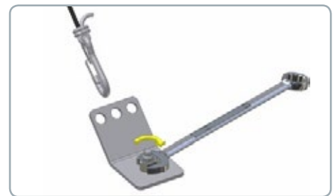
Hard ground fixing
