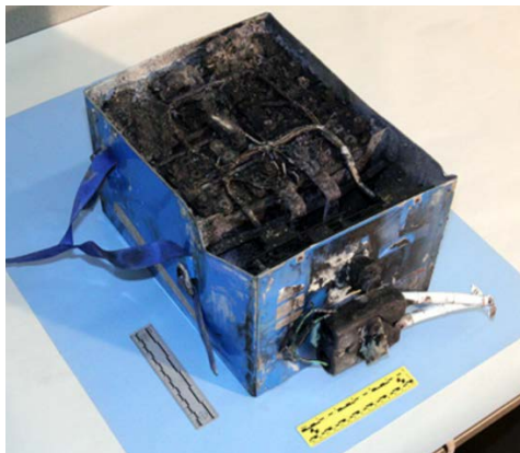
Figure 10 Boeing 787 APU Li-Ion Battery Module after Thermal Runaway (FAA/NTSB)
