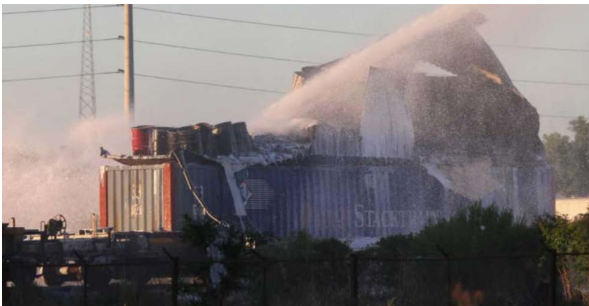
Figure 9 Explosion in Union Pacific Train Car filled with Lithium-Ion Batteries
