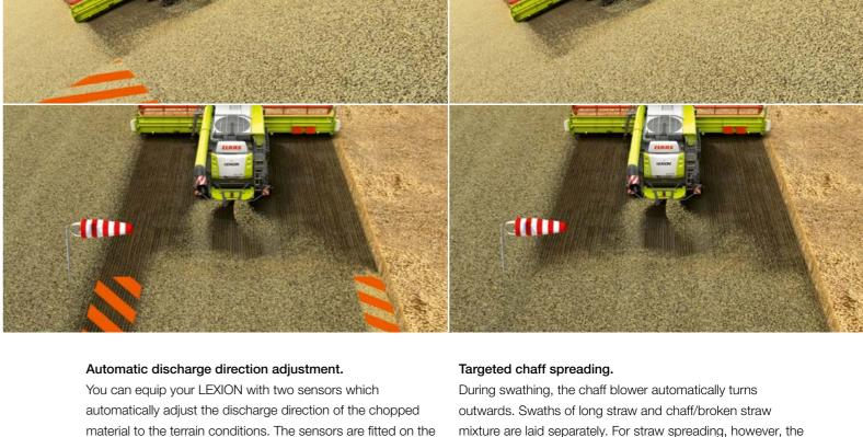
You can equip your LEXION with two sensors which automatically adjust the discharge direction of the chopped material to the terrain conditions. The sensors are fitted on the light brackets at the rear of the machine and ensure that the power spreader and deflector spread the chopped material evenly on slopes or in the event of crosswind. You set the sensitivity of this system in CEBIS.
