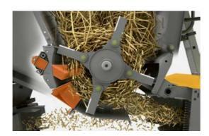
Static knife and pivoting bottom element in SPECIAL CUT chopper
