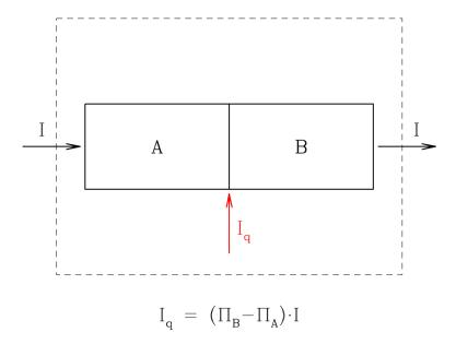
Figure 1.12: A sketch of a Peltier effect refrigerator. An electrical current I is passed through a junction between two dissimilar metals. If the dotted line represents the boundary of a thermally well-insulated body, then the body cools when  $\sqcap_{\mathcal{B}} > \sqcap_{\mathcal{A}}$ , in order to maintain a heat current balance at the junction.
