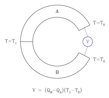
Figure 1.11: A thermocouple is a junction formed of two dissimilar metals. With no electrical current passing, an electric field is generated in the presence of a temperature gradient, resulting in a voltage  $V = V_{\rm A} - V_{\rm B}$ .
