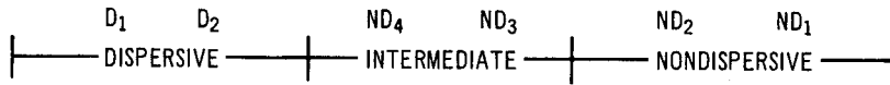
Figure 4. Typical sequence of testing and classification of test results for pinhole erosion test using 4.6-in.-long specimens
