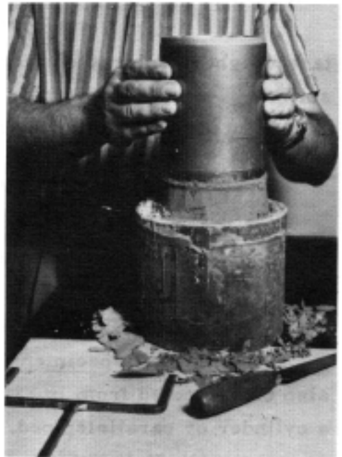
Figure 3. Determining the unit weight of a soil specimen with the volumetric cylinder (split-ring type)
