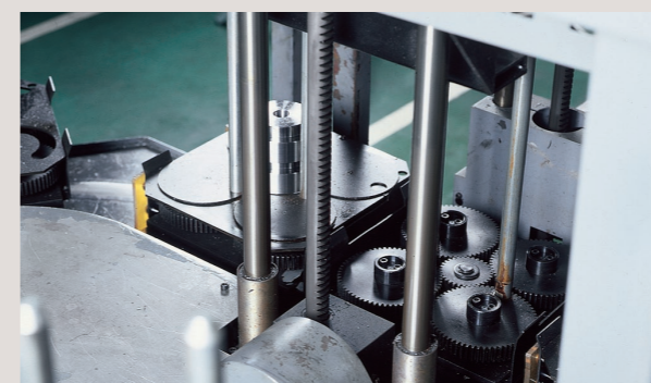
KSRO Round Rack used as a workpiece storage device (lifting/lowering table)
