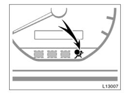
This indicator comes on when the ignition key is turned to the "ACC" or "ON" position. It goes off after about 6 seconds. This means the front seat belt pretensioners are operating properly.
