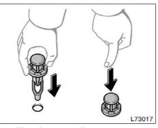
Installing the cover clips
