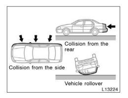
The SRS airbags are not designed to inflate if the vehicle is involved in a side or rear collision, if it rolls over, or if it is involved in a low-speed frontal collision. The SRS airbags may deploy if a serious impact occurs to the underside of your vehicle. Some examples are shown in the illustration.
