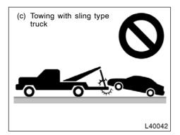
(c) Towing with sling type truck
