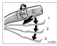
To turn on the windshield wipers, move the lever to the desired setting.
