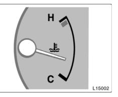
The gauge indicates the engine coolant temperature when the ignition switch is on. The engine operating temperature will vary with changes in weather and engine load.
