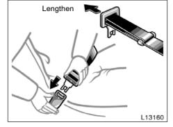
Sit up straight and well back in the seat. To fasten your belt, insert the tab into the buckle.
