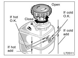
Check the fluid level through the reservoir. If necessary, add automatic transmission fluid DEXRON<sup>®</sup>II or III.
