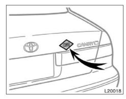
A special label is pasted close to the license plate on a CNG vehicle. Do not remove this label.
