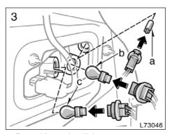
a: Rear side marker light b: Rear turn signal light c: Stop and tail light
