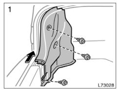
Use a Phillips-head screwdriver. Remove and install the cover clips as shown in the following illustrations.
