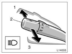
**High-Low beams**—For high beams, turn the headlights on and push the lever away from you (position 1). Pull the lever toward you (position 2) for low beams.
