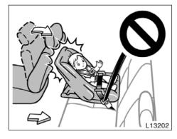
• Do not put a rear-facing child restraint system on the rear seat if it interferes with the lock mechanism of the front seats. This can cause severe injury to the child and front passenger in case of sudden braking or a collision.
