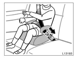
1. Sit the child on a booster seat. Run the lap and shoulder belt through or around the booster seat and child following the instructions provided by its manufacturer and insert the tab into the buckle taking care not to twist the belt.
