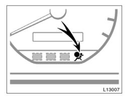
This SRS airbag system has a service reminder indicator to inform the driver of operating problems. If either of the following conditions occurs, this indicates a malfunction of the airbags. Contact your authorized Toyota CNG dealer as soon as possible to service the vehicle.
