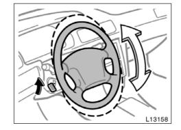
To change the steering wheel angle, hold the steering wheel, pull up the lock release lever, tilt the steering wheel to the desired angle and release the lever.
