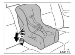
1. Run the center lap belt through or around the convertible seat following the instructions provided by its manufacturer and insert the tab into the buckle taking care not to twist the lap belt.
