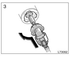
3. Install a new bulb and connector into the mounting hole.
