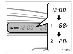
The outside temperature gauge indicates the outside air temperature.
