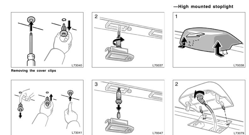
Installing the cover clips
