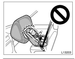
Never put a rear-facing child restraint system on the front seat because the force of the rapid inflation of the passenger airbag can cause death or serious injury to the child.
