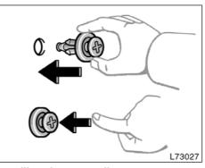
Installing the cover clips
