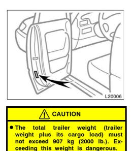
• Trailer hitch assemblies have different weight capacities established by the hitch manufacturer. Even though the vehicle may be physically capable of towing a higher weight, the operator must determine the maximum weight rating of the particular hitch assembly and never exceed the maximum weight rating specified for the trailer-hitch. Exceeding the maximum weight rating set by the trailer hitch manufacturer can cause an accident resulting in serious personal injuries.
