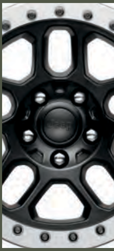
17-INCH BEADLOCK WHEEL 12-mm offset allows for larger tires. [ 77072466AB - BEADLOCK WHEEL WITH BEAUTY RING ] [ P5160154 - FUNCTIONAL BEADLOCK RING ]
