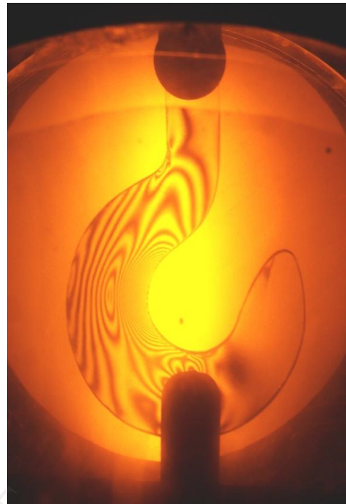
Figure9. Isochromatic fringe pattern developed in photoelastic model of crane hook
