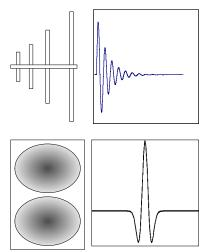
Figure 1: A log periodic antenna (upper left) has a dispersive waveform (upper right), while an elliptical dipole (lower left) has a non-dispersive waveform (lower right).
