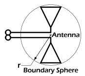
Figure 9: The boundary sphere around an antenna.
