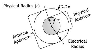
Figure 12: Physical aperture and antenna aperture.
