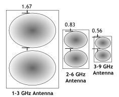
Figure 6: A family of planar elliptical dipole antennas responsive to various frequency ranges. Element size is shown in inches.
