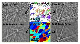
TKD map from a nanoscale SiC sample (courtesy of Dr Y Zayachuk) comparing Hough- (upper row) and PCA- (lower row) based analyses. Central panel shows an IPF map from the Hough analysis and the PCA segmentation of grains on the basis of strongest contributing pattern. Example patterns are given to the left and right showing the improvement in pattern quality achieved via MSA.
