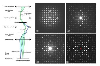
Figure 1. Simplified ray path for precession electron diffraction and experimental PED patterns (with a kinematical simulation for comparison
