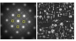
Figure 2 : Grain boundary and precipitates in a Nibased super alloy generated from an EMPAD 4DSTEM dataset. (200kV) Sample courtesy: Prof.
