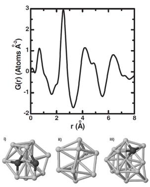
Fig.1, *Phys. Rev. B* **79**, 014203 (2009): (top) Example of a reduced density function, G(r), of an amorphous ferromagnetic  $Co_{40}Fe_{40}B_{20}$  thin film. The peak positions correspond to characteristic bond lengths in the material.
