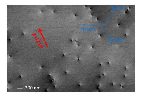
Threading dislocations in a GaN film on sapphire viewed 'end-on' using ECCI
