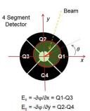
Figure 1: Segmented ADF detector illustrated with principle of DPC contrast
