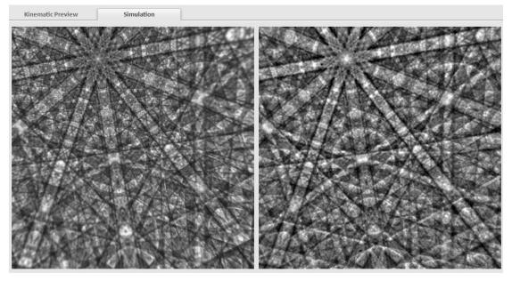
Fig.1 Kikuchi Patterns observed from a Gallium Nitride sample [2] compared to a simulation using dynamical electron diffraction theory as implemented in ESPRIT DynamicS (Bruker Nano)
