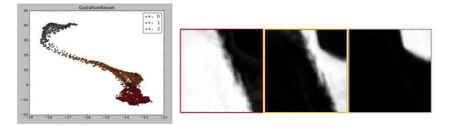
Figure 1. Clustering results from a nickel alloy studied by scanning electron diffraction.
