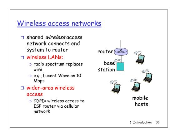
Mobile access networks use the radio spectrum to connect a mobile end system (for example, a laptop PC or a PDA with a wireless modem) to a base station. This base station, in turn, is connected to an edge router of a data network. An emerging standard for wireless data networking is cellular digital packet data (CDPD).
