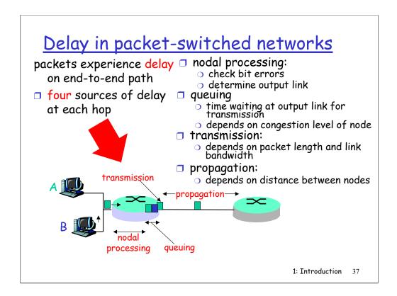
As a packet travels from one node (host or router) to the subsequent node (host or router) along this path, the packet suffers from several different types of delays at each node along the path. The most important of these delays are the nodal processing delay, queuing delay, transmission delay, and propagation delay; together, these delays accumulate to give a total nodal delay.
