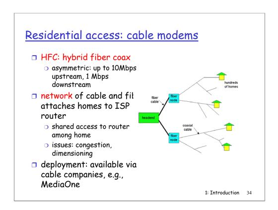
ADSL, ISDN, and dialup modems all use ordinary phone lines, but HFC access networks are extensions of the current cable network used for broadcasting cable television. In a traditional cable system, a cable head end station broadcasts through a distribution of coaxial cable and amplifiers to residences. As with ADSL, HFC requires special modems, called cable modems.
