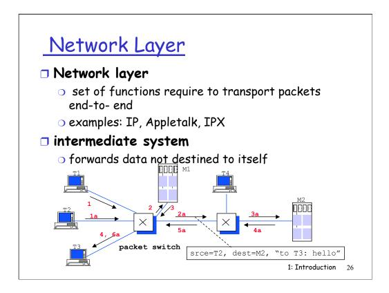
Modern networks have more than physical and data link. The **network layer** is the set of mechanisms that can be used to send packets from one computer to another in the world. There are two types of networks:
