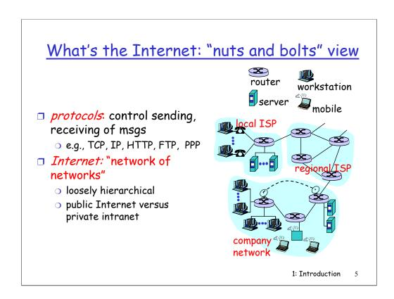
End systems, as well as most other "pieces" of the Internet, run protocols that control the sending and receiving of information within the Internet. TCP (the Transmission Control Protocol) and IP (the Internet Protocol) are two of the most important protocols in the Internet. The Internet's principal protocols are collectively known as TCP/IP.
