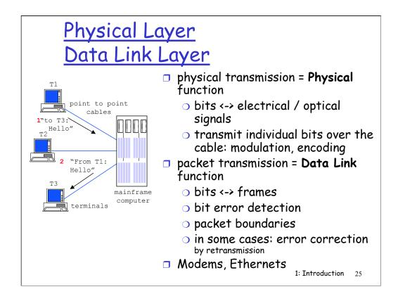
We start with the simplest, and oldest, network example: it is a mainframe connected to terminals. In that case, there are mainly two functions
