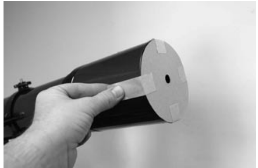
Figure 7: Because the SSDSI is so sensitive to light, an aperture mask is needed on the telescope for any imaging during daylight.
