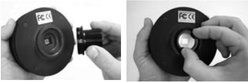
Figure 8a-b: (8a.) To install the IR filter, first remove the nosepiece by unthreading it from the SSDSI. (8b.) The IR filter then threads directly onto the SSDSI.
