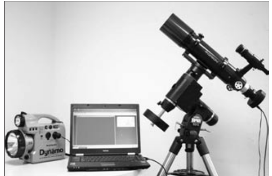
Figure 1: To use the SSDSI, a telescope, mount, computer, and 12VDC power source (for TEC usage only) are required.
