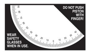
The angle is easily adjusted using the thumb screw. The built-in protractor and plumb bob on the side of the launcher give a convenient and accurate way of determining the angle of inclination.
