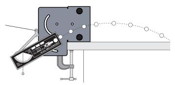
Clamp base to table. Mount launcher as shown to shoot onto table. The square nut that the Launcher pivots around should be slid to the front of the launcher. Ball is launched at table level. When you change the angle of the launcher, the launch position does not change.
