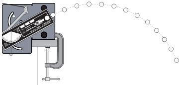
Clamp base to side edge of table. Mount launcher as shown to shoot off table onto floor at a positive or negative angle.
