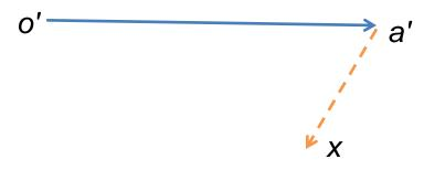
4. From point x, draw vector xb'perpendicular to A B or vector a'x (because tangential component of B with respect to A *i.e.*  $a_{BA}^t$ , is perpendicular to radial component  $a_{BA}^r$ ) and through o' draw a line parallel to the path of B to represent the absolute acceleration of B *i.e.*  $a_{B}$ . The vectors xb' and o' b' intersect at b'. Now the values
