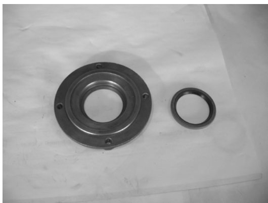
Figure 48: Bearing Cap and Lip Seal
