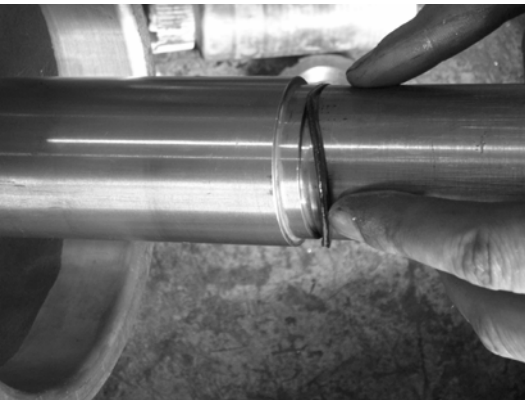
Figure 37: Installing the Quad Rings
