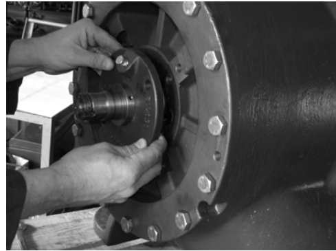
Figure 28: Removing the Gland Assembly and Sleeve
