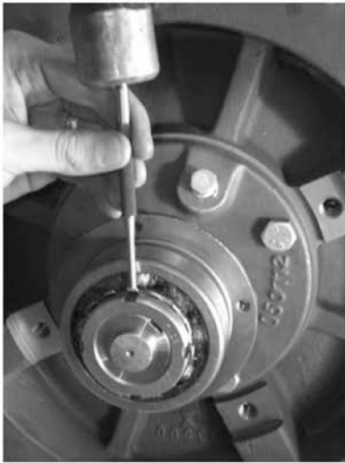
Figure 50: Installing the Lockwasher and Locknut
