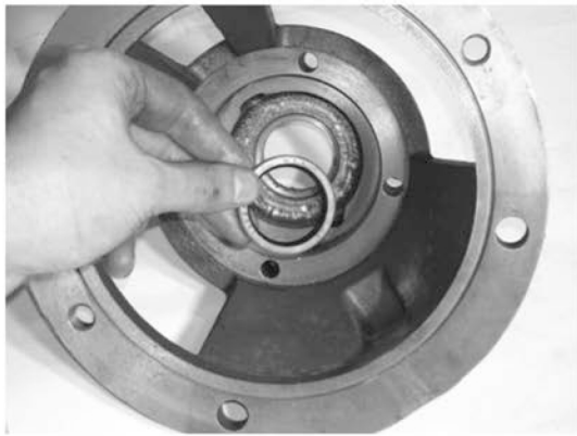
Figure 51: Bearing Bracket and Lip Seal
