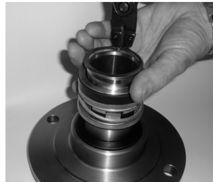
Figure 29: Mechanical Seal Head and Gland with Retaining Ring Removed
