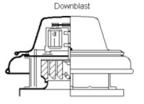
The drawing below shows a typical exhaust fan installation.
