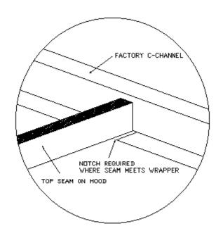
FIG. 3 TOP HOOD SEAM DETAIL
