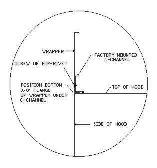
FIG. 1 WRAPPER DETAIL
