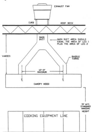
The normal requirement states that a hood and associated ductwork must have an 18" clearance from combustible materials. Since this is too great in most installations, BOCA, NFPA and the Uniform Mechanical Code have produced approved methods of protecting exhaust ducts from surrounding combustibles to reduce this clearance to 3". Please observe the method approved by local authorities governing your area.
