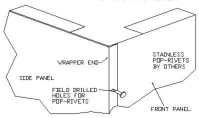
FIG.5 FRONT CORNER ASSEMBLY
