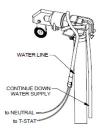
3/4" Valve Cable Heater Setup
