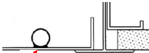
Spot contact with tubing soldered directly to metal panel
