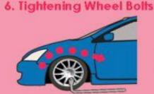
lighten wheel bolts by turning tire iron clockwise. Tahten one bolt at a time by alternating from one to the other in a "X" direction.
