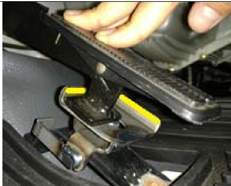
Figure 6 – View From Left Side. Yellow indicates stopper bracket flange.
