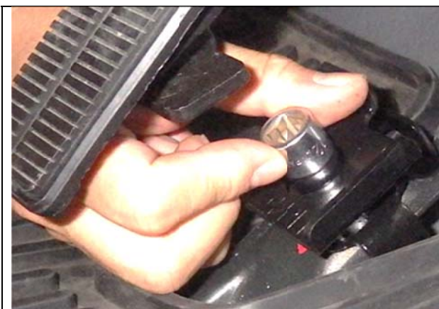
Figure 3 – Temporary Bracket Installation
