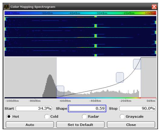
Fig. 4-4: Color mapping: the lower end of the color map is increased to fade out noise – the default straight line was also modified to highlight signal levels above -20 dBm
