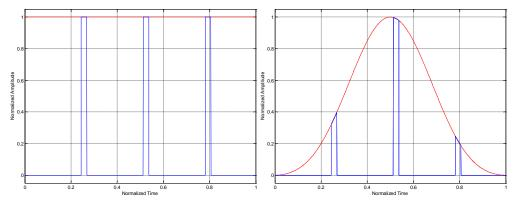
Fig. 2-3: Pulse signal in time domain. Different window functions are applied to the same signal: left - rectangular - no weighting, right - Blackman - pulses on the right and left are highly attenuated
