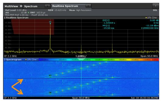
Fig. 4-3: Spectrogram with two black lines, indicating non-contiguous captures, i.e. gaps, due to triggered mode or single sweep operation
