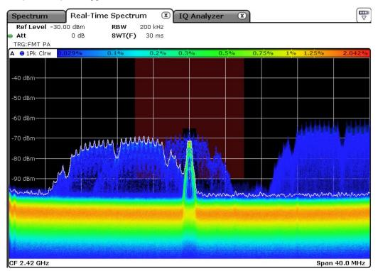
Fig. 3-2: Active FMT triggered by frequency change of a WLAN signal
