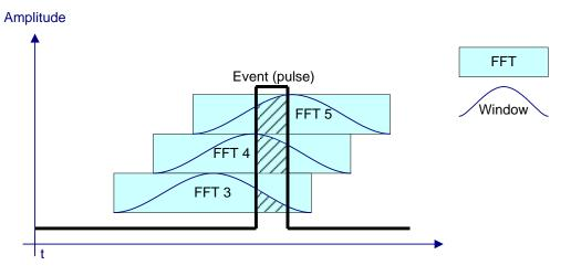
Fig. 2-7: Overlapping compensates effects resulting from windowing function
