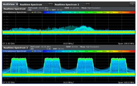
Fig. 4-6: Frequency agile DUT in the 2.4 GHz ISM band and 5 GHz band. Persistence shows signal longer than its duration
