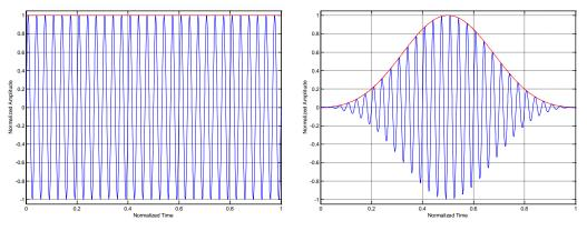
Fig. 2-2:Sine wave signal in time domain. Different window functions are applied to the same signal: left - rectangular, right - Blackman
