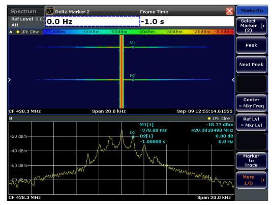
Fig. 4-5: Timing measurement with split screen spectrogram and real-time spectrum
