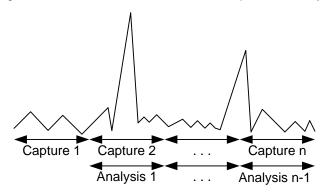
Fig. 1-2: Parallel capture and analysis as used in real-time analyzers
