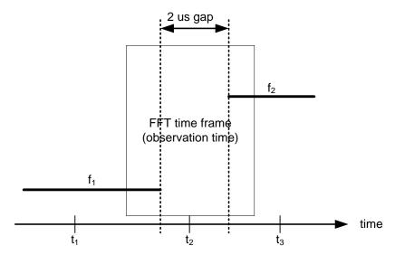
Fig. 2-8: Timing diagram of the FFT observation time example
