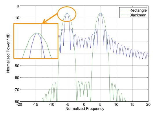
Fig. 2-4: Frequency domain view of the signal from Fig. 2-2. The Blackman window shows significantly lower spectral leakage than the rectangular window, but a wider main lobe. The inlay compares the amplitude accuracy.
