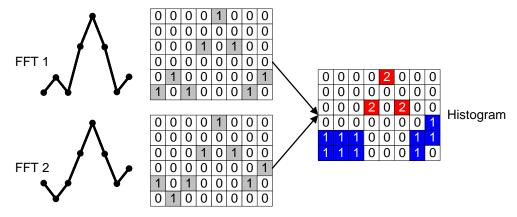
Fig. 4-8: Schematic of histogram calculation (dot style)
