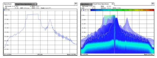
Fig. 1-3: Comparison of a Max Hold spectrum analyzer trace and a persistence spectrum trace
