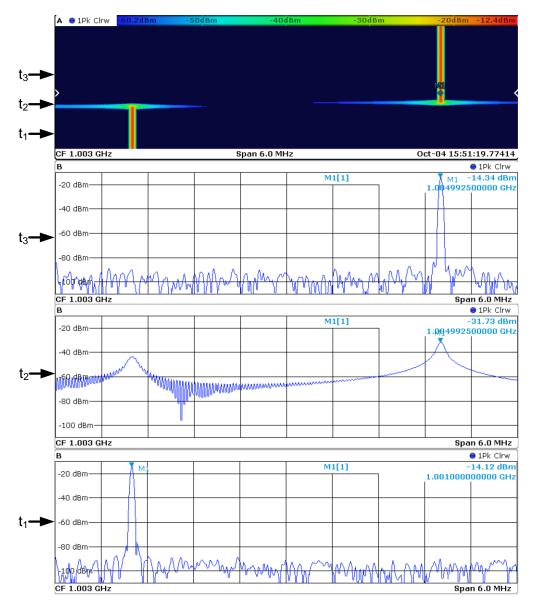
Fig. 2-9: Spectrogram showing a frequency hop. From top to bottom, the spectrum traces show frequency f2, both frequencies, and frequency f1. The trace with both frequencies results from the FFT time frame being longer than the gap between the signals.
