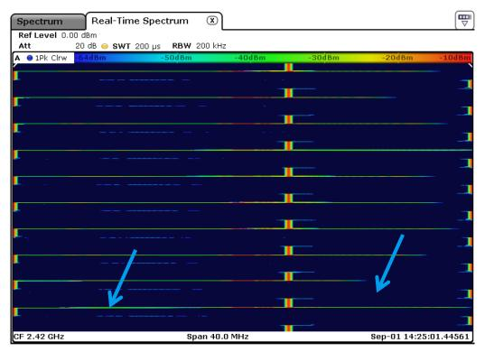
Fig. 4-1: Frequency hopper regularly hopping between 3 frequencies. First transition shows significant RF level, second transition shows almost no level during hop. Transitions highlighted by arrows.
