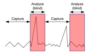
Fig. 1-1: Sequential capture and analysis as used in e.g. FFT analyzers
