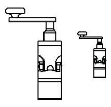
When you create a child view (Section View, Detail View, and so on), the scale of the child view can be the same as the parent view, the same as the drawing sheet, or a custom scale. This section view has the same scale as its parent view.
