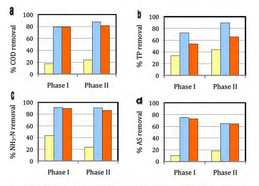
Removal by EC unit Removal by EC-SMBR process Removal by SMBR process
