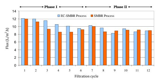
Figure 4. Average permeate fluxes from EC-SMBR and SMBR processes during the two experimental phases
