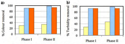
Removal by EC unit Removal by EC-SMBR process Removal by SMBR process
