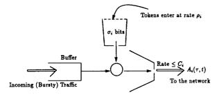
Fig. 3. A Leaky Bucket.
