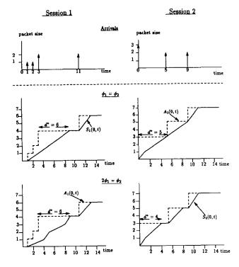
Fig. 1. An example of generalized processor sharing.
