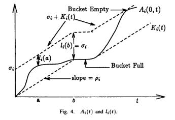
on the number of packets that can be buffered, but the *token* bucket contains at most  $\sigma$  bits worth of tokens. In addition to securing the required number of tokens, the traffic is further constrained to leave the bucket at a maximum rate of  $C > \rho$ .
