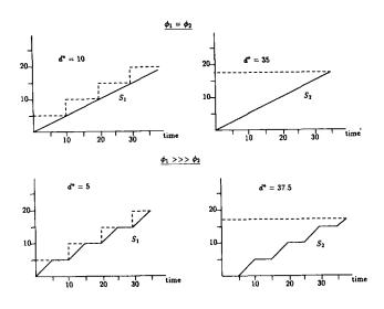
Fig. 2. The effect of increasing  $\phi_i$  for a steady session i}.
