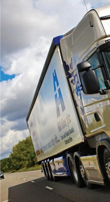
Historically, this would have led to a retest, but with resources stretched in an age of austerity, it's a case of grin and bear it. That said, the figures stack up well enough: it returned 7.89mpg, a figure built from 8.7mpg on the opening day. Day two returned 7.31mpg. With no AdBlue, the running cost is £39.39p per 100km.
