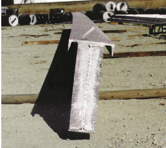
Figure 6. Distorted Asymmetric Beam
