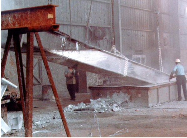
Figure 8. Progressively Dipped Beam
