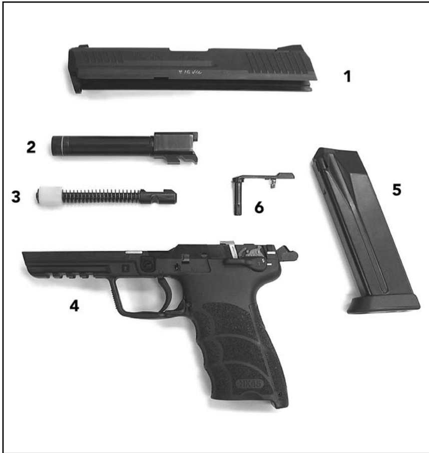
Figure 22 HK45 fieldstripped into Major Assembly Groups
