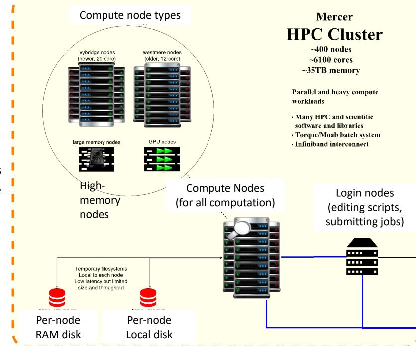
Infiniband interconnect between storage and compute
