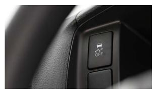
VSC (Vehicle Stability Control) helps you correct a loss of control by detecting if the vehicle is starting to skid or slide. By comparing the vehicle's direction of travel with your steering, acceleration and braking inputs it can tell if you are deviating from the intended direction. VSC then warns you, reduces engine power and controls the brakes to help you correct the situation.
