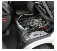
The cab forward design neatly packages the engine under the front passenger seat.
