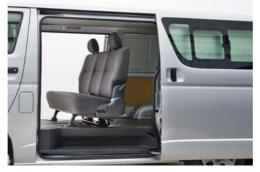
A second row seat in ZL half panel and full glass manual models provides extra seating capacity for three or can be folded for additional cargo space.
