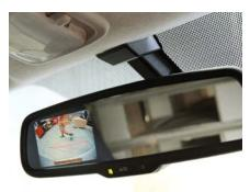
Each Hiace features a reversing camera with static guide lines and a clever colour monitor camera embedded in the rear view mirror, offering extra convenience in confined urban delivery zones and added peace of mind when reversing in residential areas.
