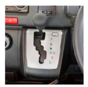
An important feature is the dash mounted gear lever that maximises interior space.
