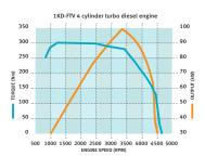
The 3.0 litre common rail turbo diesel engine is a four cylinder 16 valve DOHC design with intercooler that produces maximum torque from just 1200rpm.
