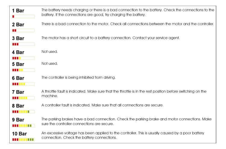
If the lights are lighting up and down in sequence it means the controller has been switched on with control knob left with power on (safety lock out to avoid runaways). Return control knob to zero for the controller to unlock.
