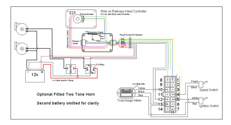
We would not recommend using sound systems that tap in to the control wires unless you can guarantee there will be no interference with the function of the iDrive unit. Stray voltage from sound systems have been known to cause controllers to power up or lock in full speed.
