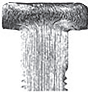
Metal flow lines of a cold-headed product
