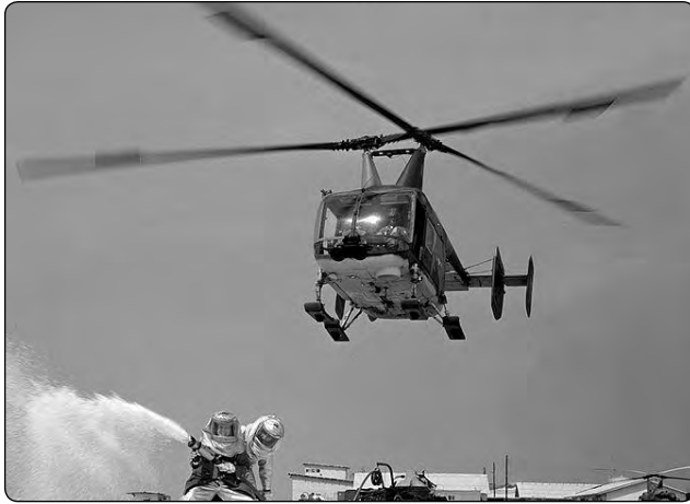
Figure 1-8. HH-43 Huskie with intermeshing rotors.
