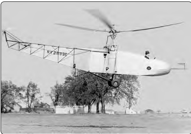
Figure 1-5. Igor Sikorsky designed the VS-300 helicopter incorporating the tail rotor into the design.
