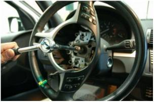
Using a socket spanner with an extension piece, remove the large bolt in the center on the wheel. This may be very tight and difficult to loosen at first.
