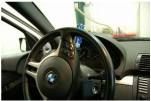
Insert a narrow screwdriver in the hole behind the steering wheel. You should feel a spring action to release one side of the airbag. Do the same on the other side to release the airbag completely.
