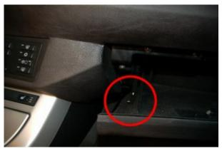
On the left side there is a plastic arm that slides down. Lift the glove box just a touch and remove the plastic rivet holding it in place. This should just slide out to the left.
