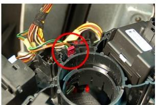
Plug in all the connectors just as they were on the old switch. Here you see the new connector for the heated wheel. Plug this into the back of the column switch.
