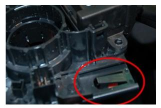
Remove the power steering stalk from the old column switch
