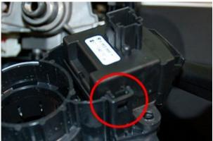
Next remove the indicator stalk and the wiper stalk. These simply snap into the column switch.
