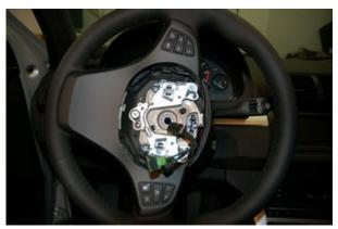
Install the new steering wheel. Be sure to align the mark on the steering wheel with the mark on the nut on the other side. Remember it will be installed sideways as shown since this is the position the old wheel was taken off in.
