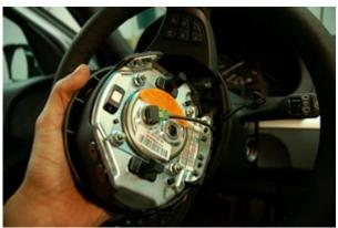
**AIRBAG MODULE, DRIVERS SIDE** (AS SHOWN IN PIC ABOVE)
