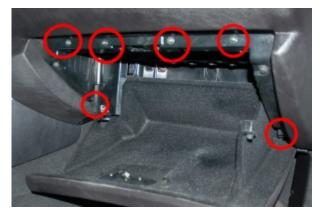
Remove all the screws as shown in the pic. The one on the bottom right is tricky to get to.
