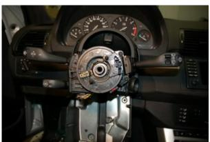
You should now be able to remove the top and bottom plastic steering column panels as shown. The top and bottom snap into each other and there are no additional screws to take them apart.
