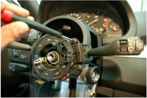
Using a small torx screwdriver, remove the 4 screw holding the steering column switch.
