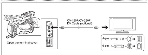
When connecting the camcorder to a monitor TV that supports DV, you may need to carry out a procedure on the TV to recognize the camera. Refer to the instruction manual of the TV or monitor. • If necessary, turn on the DV conversion and select whether to convert a tape recorded in HD to SD with the following procedure.
