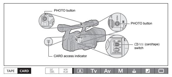
1. Turn the POWER dial to a recording program and move the 💷/📼 (card/tape) switch to 🖫.
