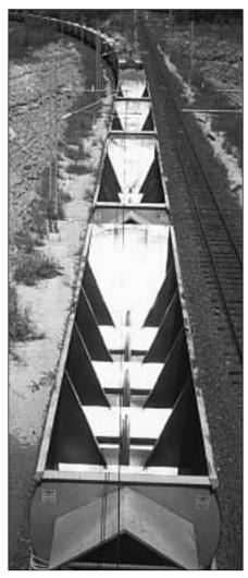
Rail coal carriers fabricated from stainless steel.
