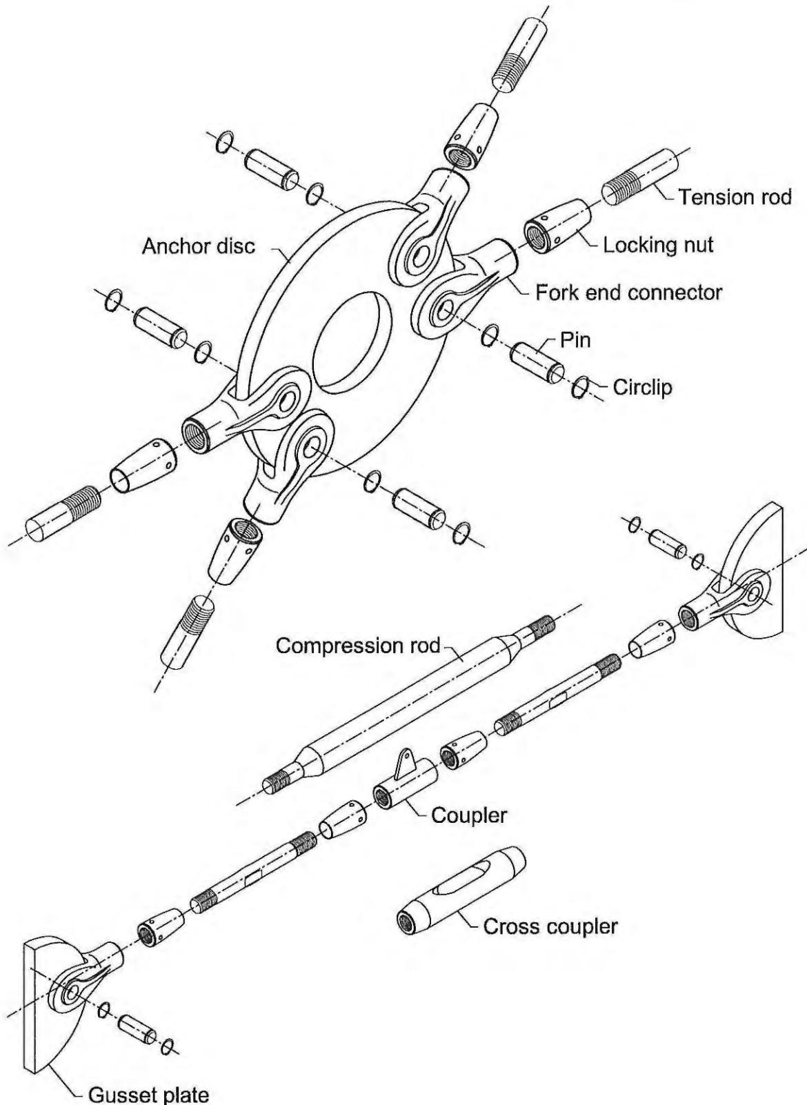
HALFEN Tension Rod System DETAN-E
