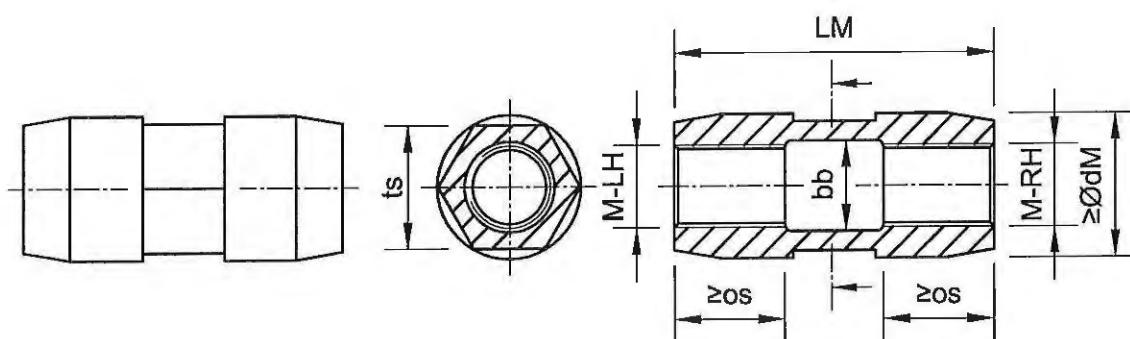
Minimum screw-in length of the tension rod = om - oj according to Annex B3
