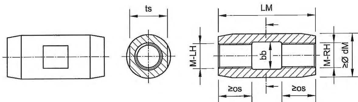
Minimum screw-in length of the tension rod = om - oj according to Annex B3
