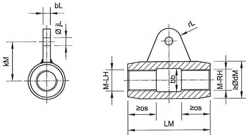
Minimum screw-in length of the tension rod = om - oj according to Annex B3
