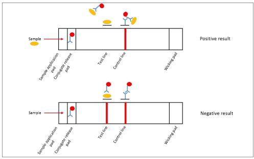
Figure 3. Competitive assay format. A positive result is seen when the analyte becomes bound to the detection antibody and therefore cannot bind to the antigen which has been immobilized at the test line. The antibody which has been immobilized at the control line will recognize the detection antibody, producing a colored line to indicate that the lateral flow assay has performed as expected.
