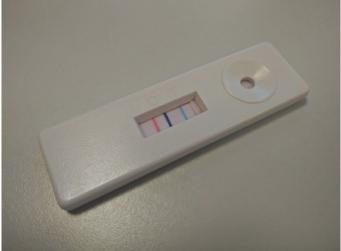
Figure 7. Multiplexed lateral flow immunoassay using Innova Biosciences' latex beads. Latex beads of three colors have each been conjugated to a different antibody or protein.
