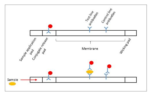
Figure 1. Schematic representation of a typical lateral flow assay. The antigen is illustrated in yellow.
