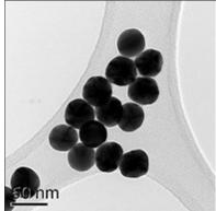
Figure 5. TEM image of 40nm colloidal gold, demonstrating the uniform spherical shape and narrow size distribution.
